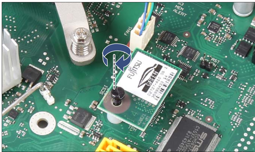
Figure 132: Securing the TPM board
